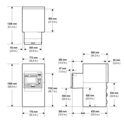
**Note:** Overall depth dimension includes the door lock. Overall width dimension includes the top door hinge.
