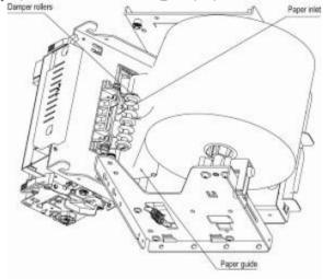
Slide the cut end of the paper roll into the paper inlet being careful to feed the paper underneath the damper rollers.
