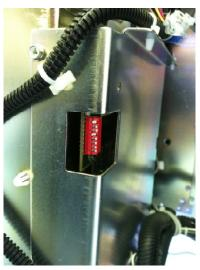
This is the secondary cash dispenser dip switch settings. Position numbers 1 and 4 are the only switches in the "closed" or "on" position.
