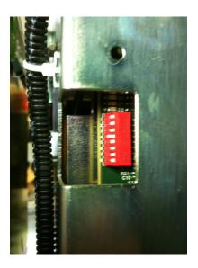
This is the primary cash dispenser dip switch settings. Position number 4 is the only switch in the "closed" or "on" position.
