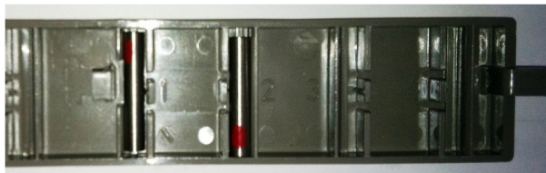
Type 1 cassette magnet configuration
