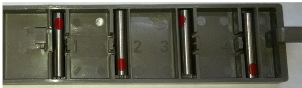
Type 4 cassette magnet configuration
