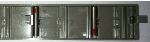
Type 3 cassette magnet configuration
